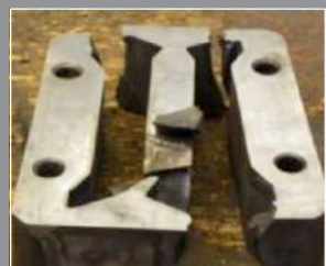
D2 / 1.2379 at 60 HRC crack after 10,000 shots
