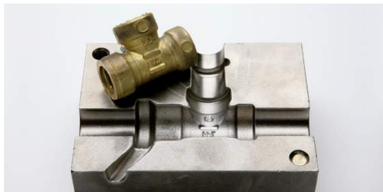
Top - Aluminium die casting. Toolox 44 offered faster manufacturing and good surface polish. Bottom - Brass die casting. Toolox 44 replaced QRO 90 to save time and material cost.
