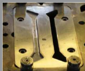
Toolox 44 + Nitriding 250,000 shots and running
